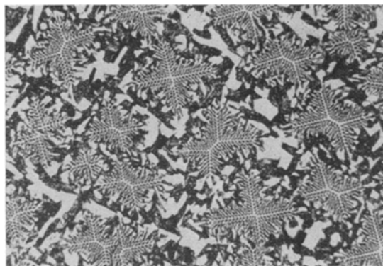
Figure 4 Micrograph of a transverse section of a unidirectionally solidified rod with an excess of \text{TiO}_2 ( \sim 1\frac{1}{2} \text{ wt } \% ) showing four finned spinel dendrites in cells, \times 100 .
